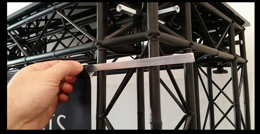
Attach top clips as shown. Clips should secure over the fabric and aluminum profile bar. Once clips are in place, snap the open end over the bottom of the module so that the graphic hangs freely. Please note: Each kit contains enough top and bottom clips to secure all graphics. While there is no required amount of clips per graphic, larger graphics will require more clips than smaller graphics to secure in place.
